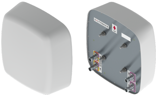
4-Port directional panel antenna covering 617-960, 1695-2690 & 3300-4200 MHz
