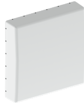
698-960, 1695-2690, 3300-4200 and 5150-5925 MHz 10-Port 30x30 Pattern Directional Panel Antenna
